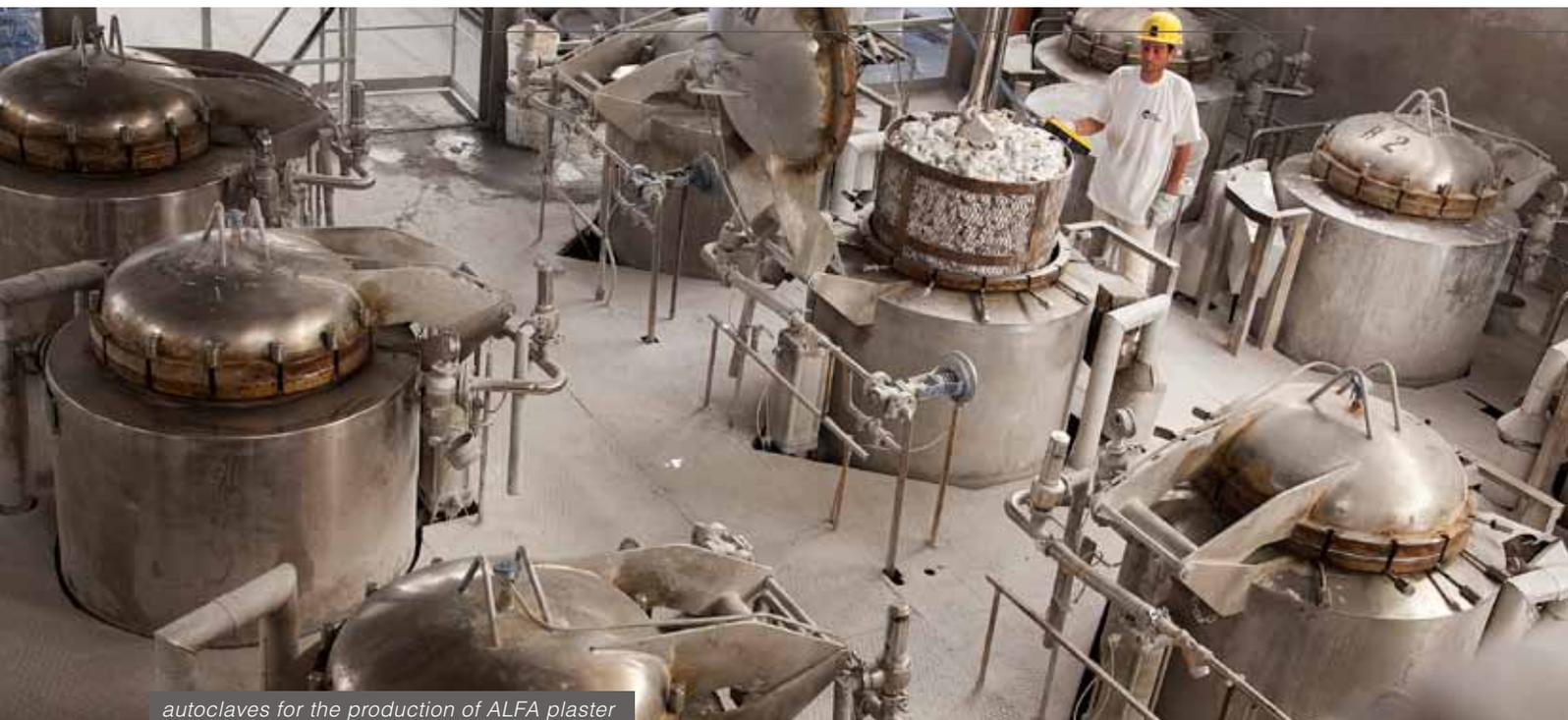
*autoclaves for the production of ALFA plaster*
